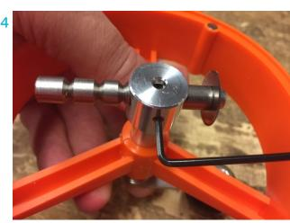
4. When you have selected the size you wish to cut, tighten the small screw in the side of the cutter arm.
