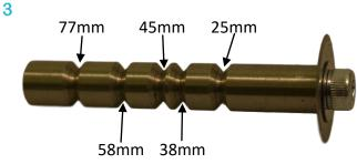
3. Look through the small hole on the bottom of the cutter arm to select the correct ridge.Each ridge will cut a different size of circle, as shown in the image 3.
