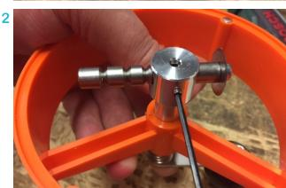
2. Use the Allen key to loosen the small screw in the side of the cutter arm. The cutter arm should now move side to side.
